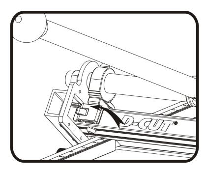
When the cutter is not in use, you need to keep the blade in a close position for the safety.
